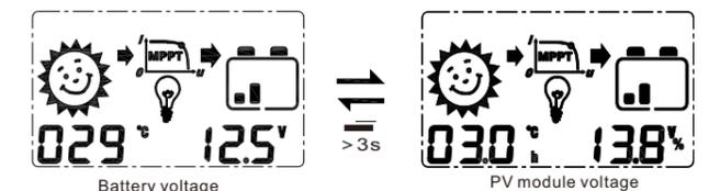
In the main loop of the battery voltage interface long press **-** button, Switch to display solar array voltage ( The % symbol serves as a distinction ) and internal temperature of the controller (The letter h serves as a distinction)
