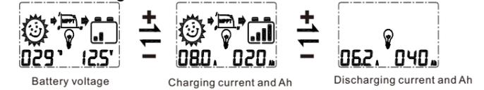
In the main loop interface, press the **+** or **-** button to enter the browsing mode, and long press the button **+** to enter the secondary browsing interface.
