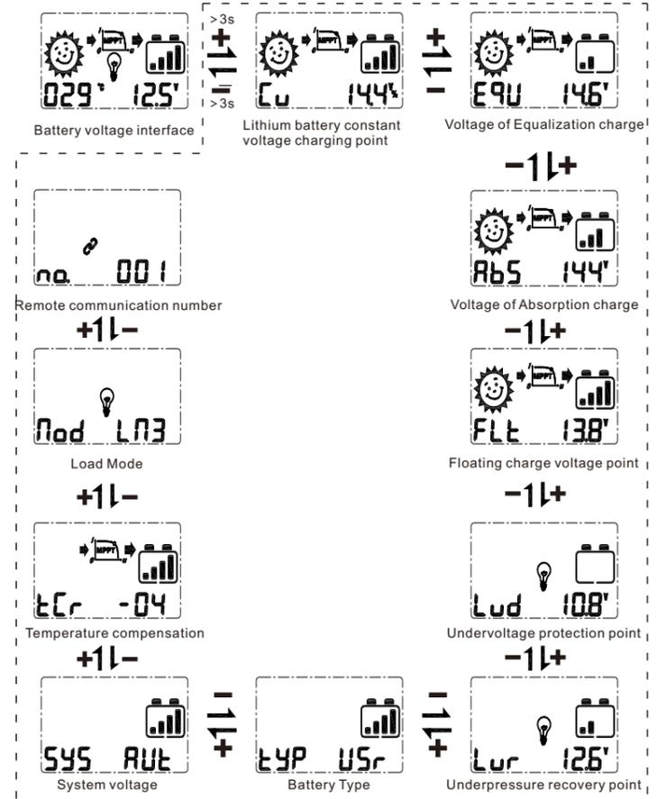
Long press the **+** button in the main loop of the battery voltage interface to enter the secondary browsing interface, short press the **+** or **-** button switch to the secondary browsing interface, long press the **+** button to enter the setting interface, short press **+** or **-** button to set the parameters and long press **+** to save .It will automatically exit the secondary browsing interface without doing anything for 20 seconds.
